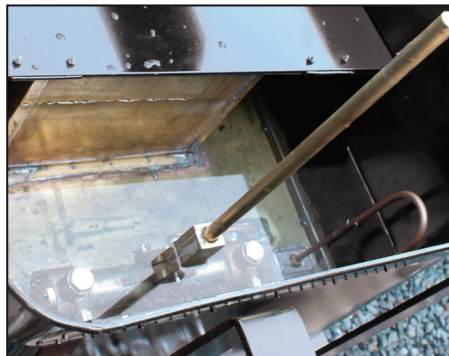
Water pump mounted in Forney bunker
